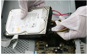
4. Place the HDD on the bottom of the device and then fasten the screws on the bottom to fix the HDD.
