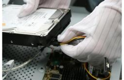
3. Connect the power cable to the HDD.
