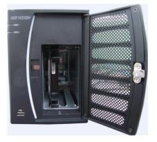
5. Repeat the above steps to install other hard disks onto the NVR. After having finished the installation of all hard disks, close the front panel and lock it with the key again.
